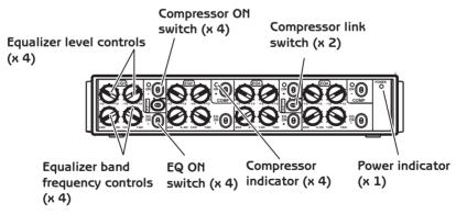
**Equalizer level controls (per channel)** Each channel has two equalizer level controls, which allow signals in the selected fre-
